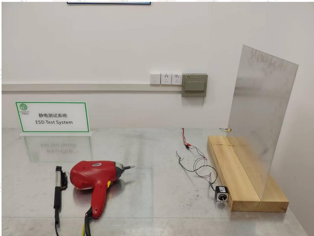
Photographs 2: Set-up for Electrostatic discharge (ESD)
