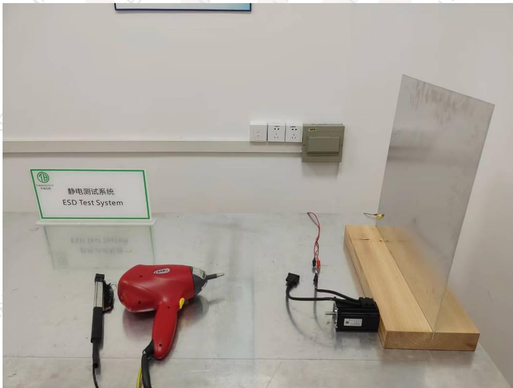
Photographs 2: Set-up for Electrostatic discharge (ESD)
