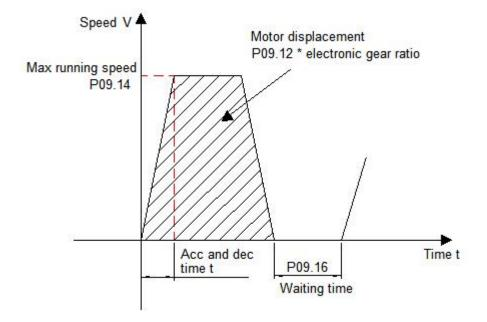
According to the above settings, the actual running curve of the motor is shown in the figure below:
