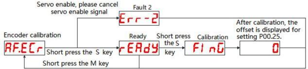
• Note: When using this operation, please disable the servo enable signal.
