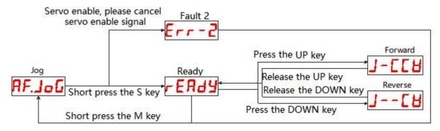
• Note: When using this operation, please disable the servo enable signal.
