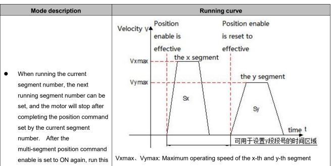
The segment number is determined by the IN terminal logic
