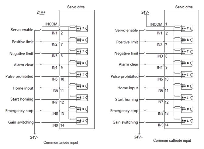
Take IN1 as an example, the wiring example is as follows:
