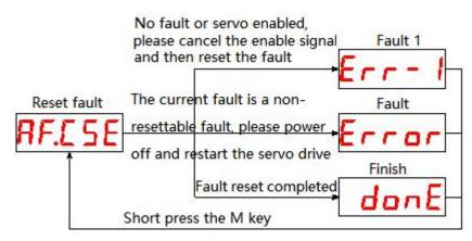
Note: When using this operation, please disable the servo enable signal, otherwise the fault information cannot be reset.
