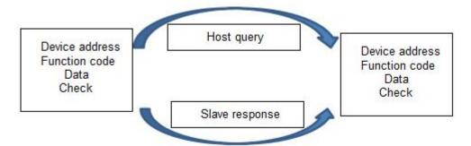
• Note: The communication data frame structure of this servo drive adopts RTU mode.
