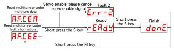
Note: When using this operation, please disable the servo enable signal, otherwise the fault information cannot be reset.
