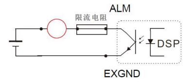
The red circle in the figure represents the switching load, which is generally used for relay or optocoupler input.
